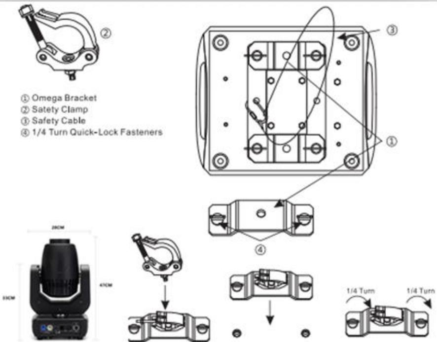
Regardless of the rigging option you choose for your LED Moving Head, always be sure to secure your fixture with a safety cable. The fixture provides a built-in rigging point for a safety cable on the hanging bracket as illustrated above. Be sure to only use the designated rigging point for the safety cable and never secure a safety cable to a carrying handle.
