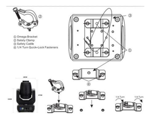
Regardless of the rigging option you choose for your LED Moving Head, always be sure to secure your fixture with a safety cable. The fixture providers a built-in rigging point for a safety cable on the hanging bracket as illustrated above. Be sure to only use the designated rigging point for the safety cable and never secure a safety cable to a carrying handle.
