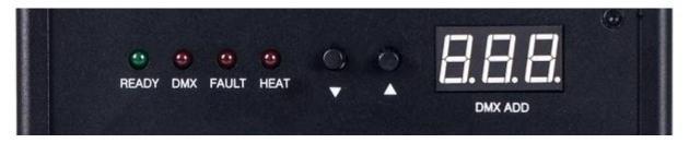
**READY:** After set the first channel(240-255 pre-heat ON) for about 5 minutes, when the "READY" green light turns from flash light to continuous light, it indicates that the machine is ready to work.
